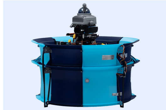
Fig. 1. Our coaxial and dual-ducted UAV, named HALO.
