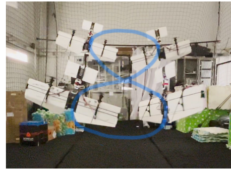
Fig. 7. The overlaid snapshots of Hong He when it tracks a 3D figure-of-eight trajectory with continuous yaw rotation.
