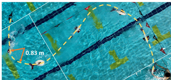
Fig. 17. Aerial view of the S-curve experiment. Snapp swims from the end of figure-8 and completes the S-curve to return to the starting point of the experiment.
